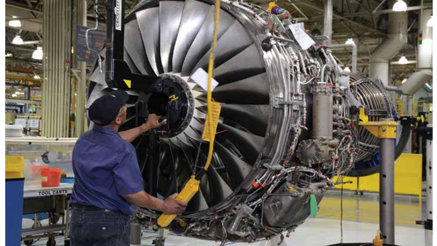
Mechanic overhauling engine at an Aftermarket Repair Shop. Pratt & Whitney Aftermarket and Sustainment Engineering group provides innovative aftermarket repair strategies for various jet engine hardware.
