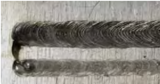
Laser weld pattern on Al3003-H14 sample.
