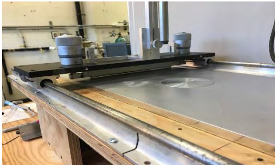
Apparatus of experiments with build plate and metal blade
